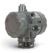
Electro-Pneumatic (I/P) Transducers convert an electronic signal to a pneumatic signal. They are routinely used in control loops that require an electronic control signal from a programmable logic controller or distributed control system to be converted to a usable pneumatic signal for operation of a control valve.
