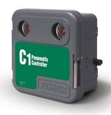
Pneumatic Controllers are mechanical devices designed to measure temperature or pressure and transmit a corrective air signal to the final control element. Bourdon tubes, bellows, temperature elements, or displacers are used as the sensing elements. The power supply and output of a pneumatic controller is compressed air or natural gas. ▶ 4194 | 4195K | 4196 | 4660 | C1 | DPC2K
